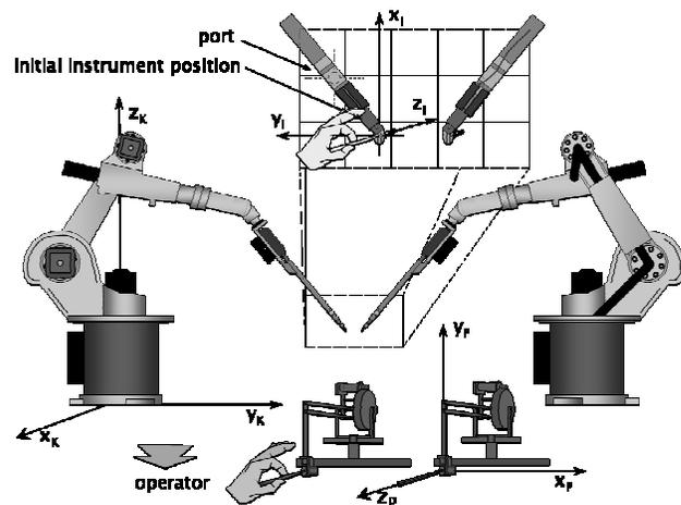
Figure 1. Telemanipulated surgical system.
