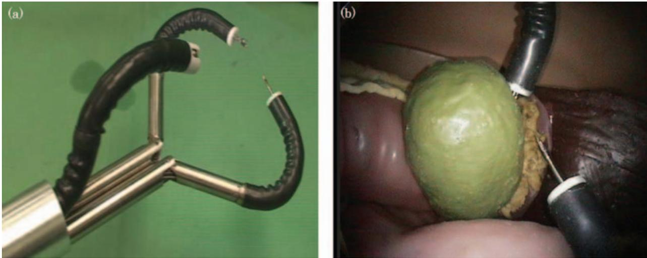
Figure 4. Application of the HVSPS for NOTES cholecystectomy: a) HVSPS manipulators in triangulated configuration with the flexible endoscope R-Scope (Olympus, Japan) b) Grasping of the gallbladder: first application of the scissors in cholecystectomy (ELITE)
