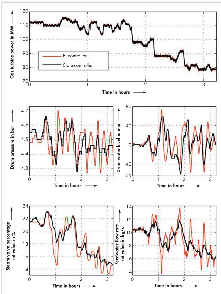
Fig. 5. Comparison between PI controller (butterfly valve) and state controller (steam turbine valve) under normal operation of the gas turbine.
