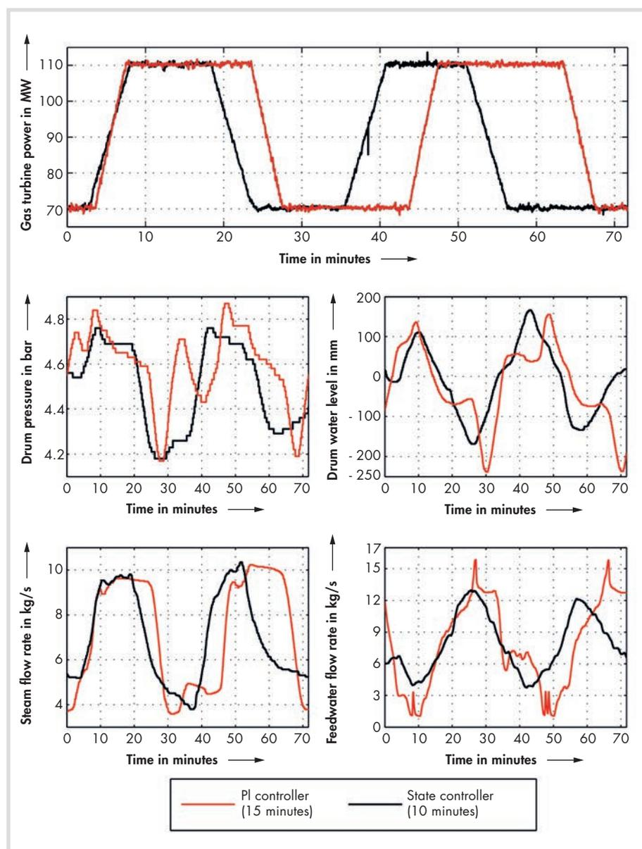
Fig. 6. Performance comparison between controllers against the prequalification curve for secondary grid control.
