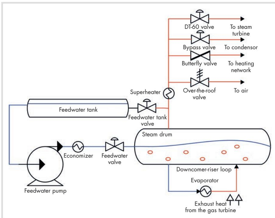
Fig. 1. Steam generation process using the steam drum.
