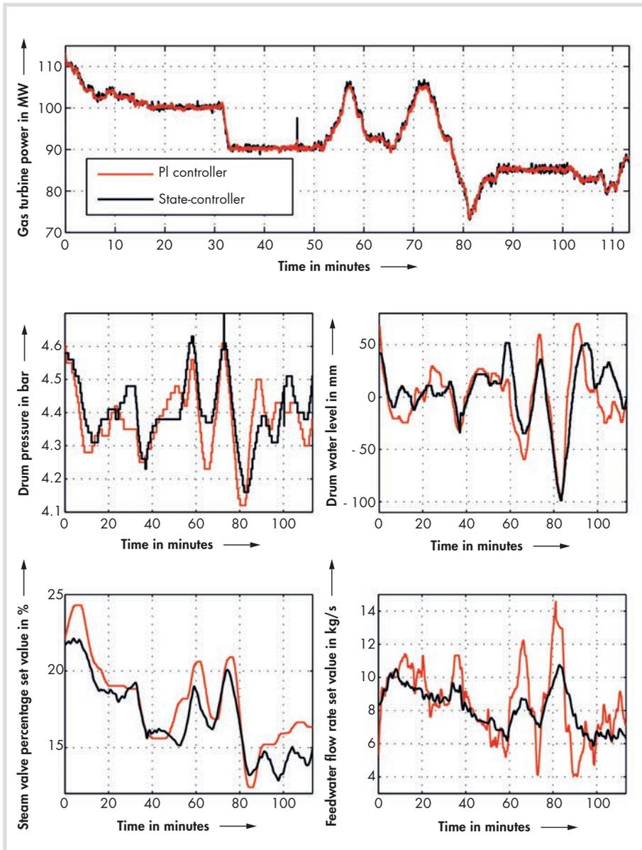
Fig. 4. Comparison between the PI-controller and the state-controller under normal operation of the gas turbine using the butterfly valve.
