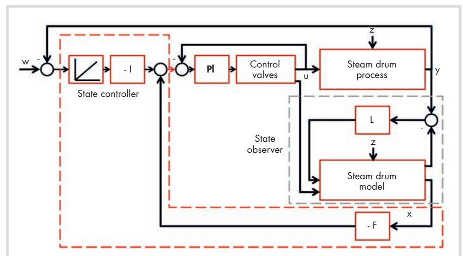
Fig. 2. Extended concept of state space control.
