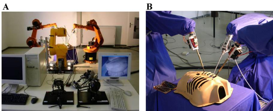
Fig. 1. Experimental platform: (A) An overview. (B) Training thorax with two haptic instruments and one camera port.
