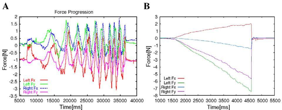
Fig. 2. Occurring forces while handling a surgical thread (Ethicon Prolene® 7/0). (A) Winding the thread. (B) Breaking the thread.
