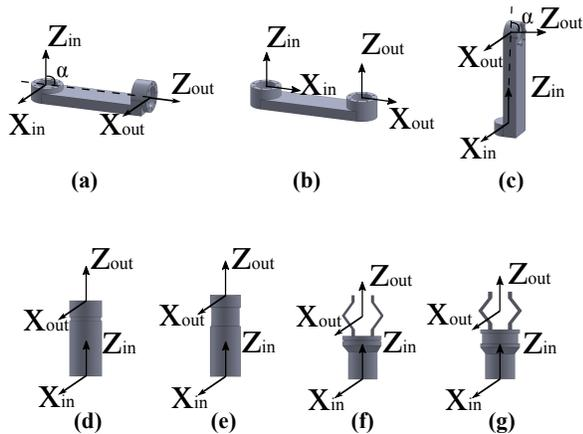
Fig. 3. Basic modules used in this study, (a)  $\alpha = 90^\circ$  link module, whose length is along the  $y$  direction of the previous coordinate system (L1), (b)  $\alpha = 0^\circ$  link module (L2), (c)  $\alpha = 90^\circ$  link module, whose length is along  $z$  direction of the previous coordinate system (L3), (d) rotational joint module (J1), (e) prismatic joint module (J2), (f) rotational end effector module (EE1), (g) prismatic end effector module (EE2)
