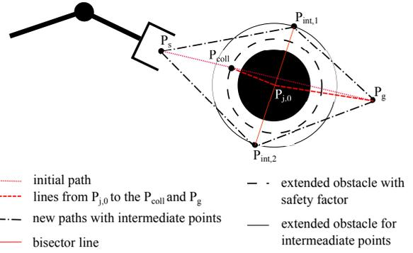
Fig. 2. Schematic diagram of the obstacle avoidance algorithm.
