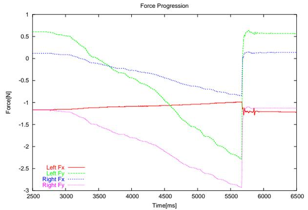
Fig. 8. Breaking Ethicon 7/0 by normal pulling
