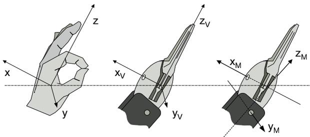
Fig. 4. Virtual Instrument Definition
