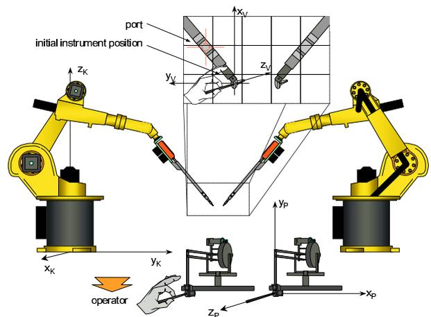
Fig. 3. Schematic System Overview
