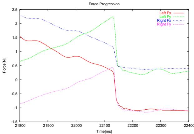
Fig. 7. Accidentally breaking a thread during winding
