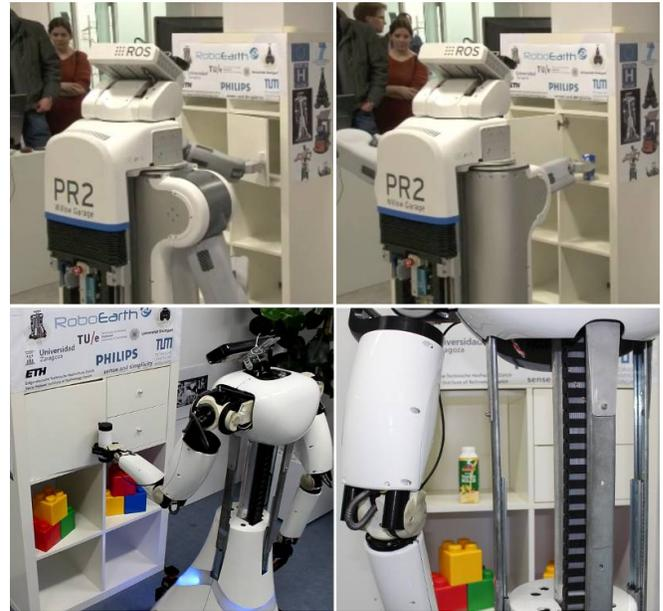
Fig. 4. A PR2 and an Amigo robot performing the same *serve drink* task in similar mock-up hospital rooms at two different locations. Both robots re-use knowledge stored in RoboEarth and use its map service for instantly being able to localize and navigate.
