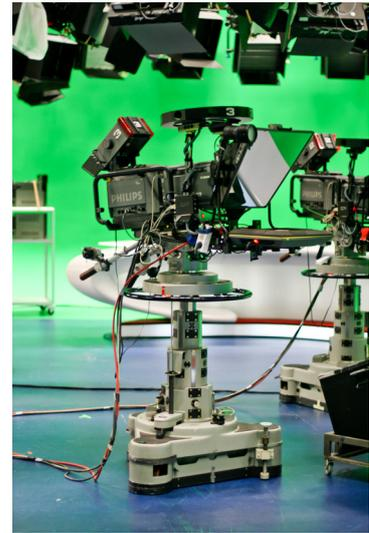
Figure 2.9: Commonly used TV Camera on a movable stand for virtual reality productions.
