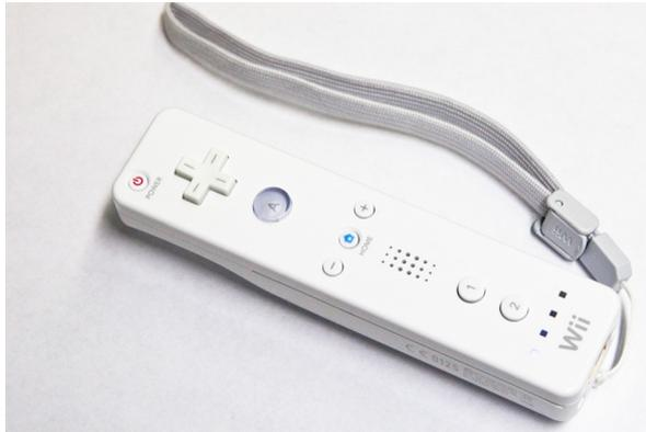
Figure 5.12: The WiiMote is a cheap and easily interfaceable Bluetooth device, that people intuitively know how to use.
