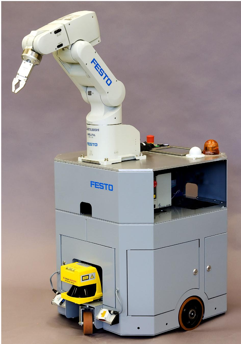
Figure 4.12: The F5-S mobile robot platform. Photo: Festo Didactic.
