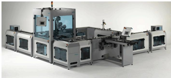
Figure 6.11: Changeable Factory made of Festo MPS modules. Photograph: Festo Didactic.
