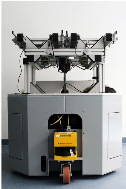
Figure 4.6: Front view of the F5 robot. Noteworthy is the 180° Leuze laser range finder.
