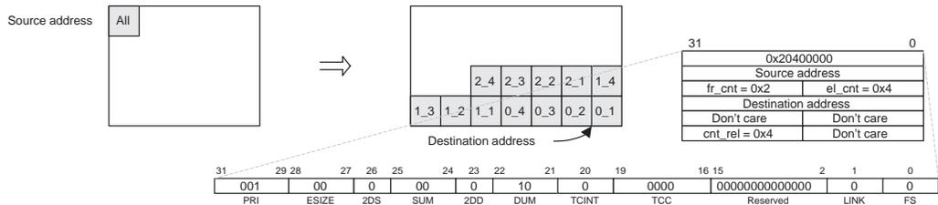
Figure A-4. Element Synchronized 1-D (SUM=00b) to 1-D (DUM=11b)
