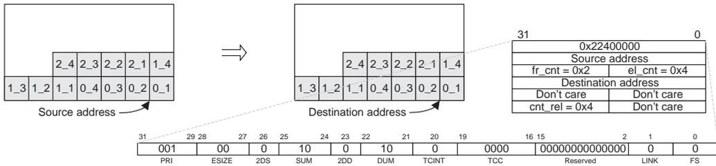
Figure A–12. Element Synchronized 1-D (SUM=10b) to 1-D (DUM=11b)
