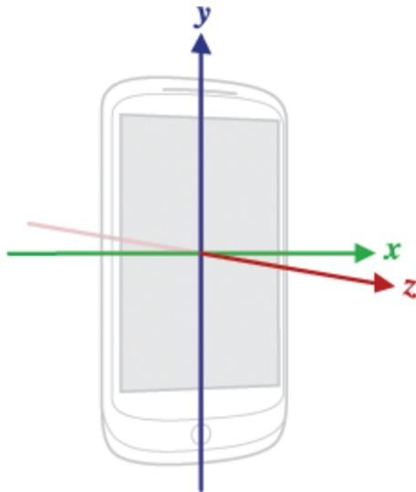
The orientation sensor lets you monitor the position of a device relative to the earth's frame of reference (specifically, magnetic north)
