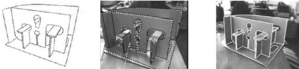
The RAPID Algorithm has been developed by using the idea above described: minimize SSD between expected and measured edge points along the normal (nearest neighbor only).
