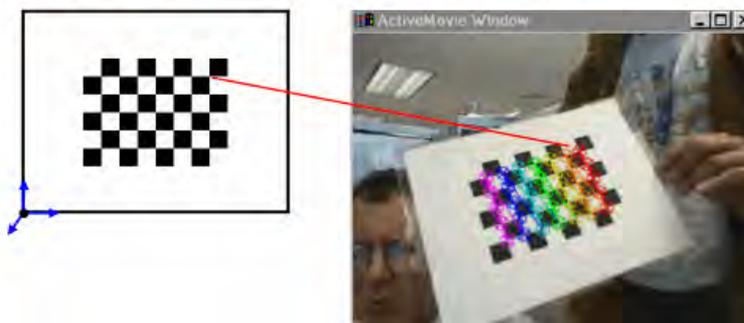
The algorithm finds both  $\mathbf{k}$  and the chessboard poses  $\mathbf{s}_1, \mathbf{s}_2, \dots, \mathbf{s}_N$  given 3D-2D point correspondences, from the chessboard model to the image.
