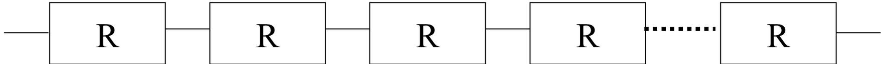
All  $n$  components above need to work such that the series assembly (system) is functioning.
