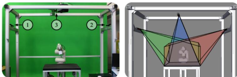
**Figure:** Setup of HRC space with sensing from multiple Kinect sensors: Lenz et Al., 2012, Fusing multiple Kinects to survey shared Human-Robot-Workspaces
