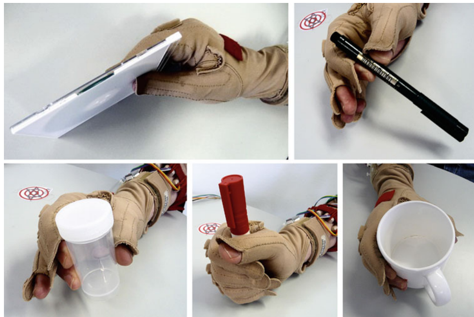
Fig. 3 The five objects while being grasped by a subject: (left to right) flat grasp, pinch grip, tripodal grip, small power grasp and large power grasp. Notice that the subject never pronates and/or supinates the forearm, as instructed
