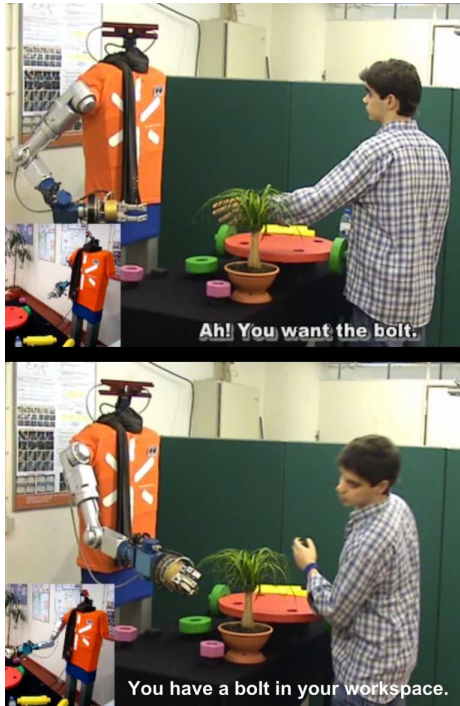
Figure 2. Example of the goal inference (top) and action selection (bottom) capacities which are implemented by the dynamic field architecture. The robot uses speech to communicate the results of its reasoning about the behaviour of the teammate.
