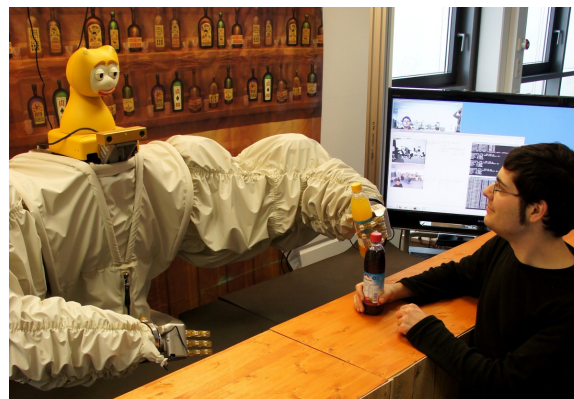
Figure 1: The robot bartender of the JAMES project uses head pose estimation to infer the state of interaction of human customers in a multi-party bar scenario.
