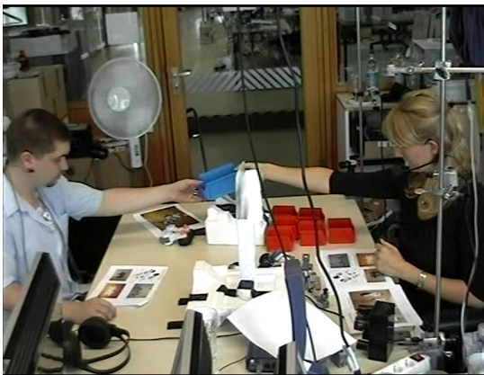
Fig. 1. Experimental setup for the MuDiS human-human experiments: the experimenter on the right enacts a “robot” that is able to hand over LEGO pieces to the experiment participant, who assembles the pieces according to a given assembly plan.
