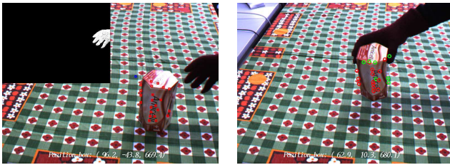
Fig. 6: Contact detection and object tracking. Left : The tracking is initialized after the contact detection between the hand and the region of interest. The small red boxes are the valid features, whereas the blue ones are the deleted features, which are not on the box. The top left corner of the image shows the position of the hand, when the contact occurs. Right : Example of features during the tracking. The tracked features are shown in red, the assumed position of the lost features are drawn in green.
