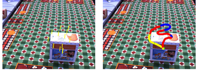
Fig. 9: Rotation, translation and speed of the object (Seq. 7). Left : The development of the rotated and translated normal vector of the table is shown in green. Right : The development of the speed along the trajectory is shown in different colors: green = no movement, yellow = slow movement, red = movement, blue = fast movement.
