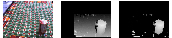
Fig. 5: Results of plane subtraction. Left column : Original color image. Middle column : Disparity image of the color image on its left. Right column : Remaining object in the disparity image after the plane subtraction.
