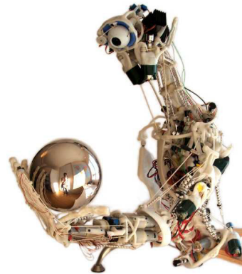
Fig. 1. Prototype of the anthropomimetic [10] robot ECCE-I [11] developed within the EU-funded project ECCEROBOT [12]. The skeleton is hand-crafted using polymorph—a caprolactone polymer—which can easily be molded. The human muscles are imitated by elastic, tendon-driven actuators comprising a DC motor and gearbox in series with a kite line and shock cord as tendon.
