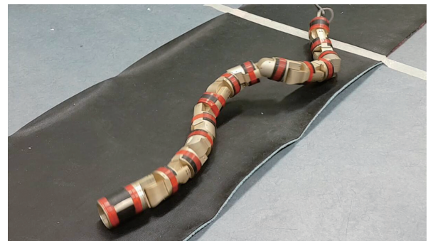
Fig. 1: The snake-like robot with a module design. Each joint axis is orthogonal to its neighbors with a rotation range of \pm 90^\circ .
