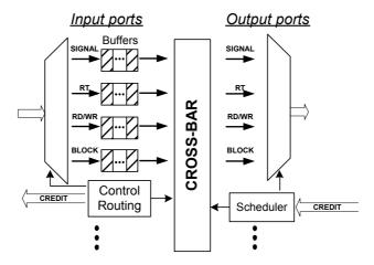
Figure 3. QNoC Router Architecture
