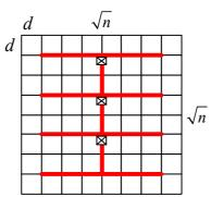
Figure 7. Bus segmented into  $\sqrt{n}/2$  segments – interconnecting n communicating modules
